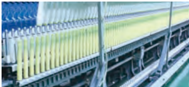
Middle-peg system accommodates large-diameter bobbins
