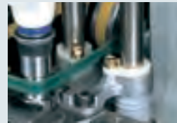
Sealed lifting pillar
