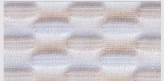
Example of weaving with yarns having a 12-times difference in yarn count Weft yarns used: P900d, cotton Ne6, cotton Ne60, P75d
