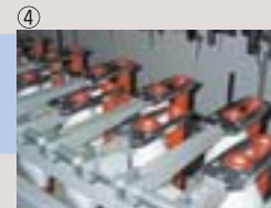
Forks simultaneously grasp full and empty bobbins
